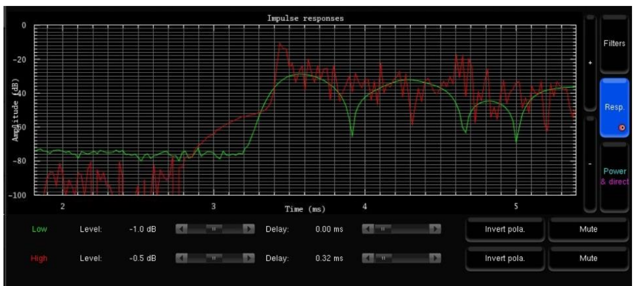
Figure 87: measured impulse response of both drivers
